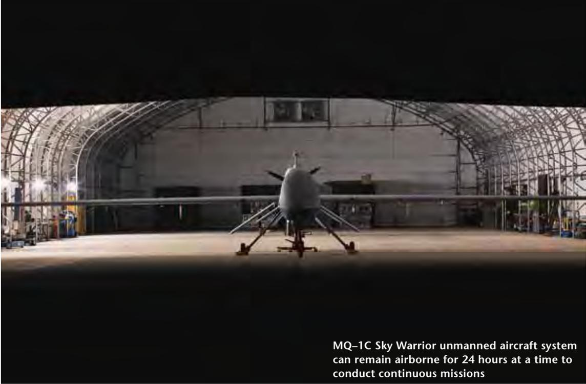
MQ-1C Sky Warrior unmanned aircraft system can remain airborne for 24 hours at a time to conduct continuous missions
